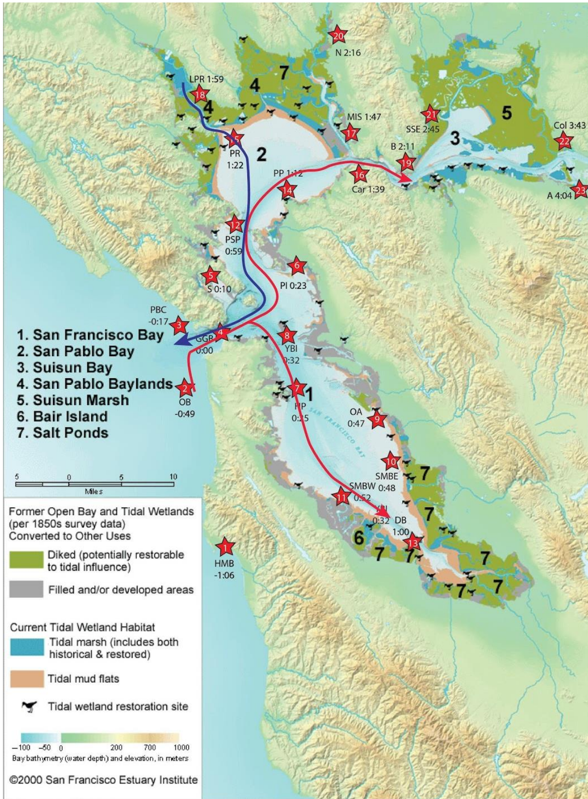
Tidal wetlands from the 1850s and 2000. Red stars are tidal locations that correlate with preceding table and indicate the time difference between high tides at this location and those at the Golden Gate Bridge. For example, In Half Moon Bay (HMB), high tide arrives 1 hour and 6 minutes BEFORE it reaches the Golden Gate Bridge. The tide flood current migrates north into the bay and then splits. It arrives at Yerba Buena Island (YBI) 32 minutes AFTER it reached the Golden Gate Bridge. Modified from original image produced in 2000 and used with permission from San Francisco Estuary Institute.
