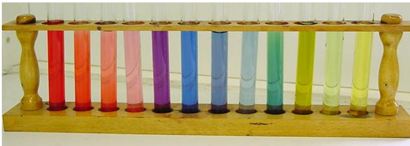
pH color chart for red cabbage pH indicator. Red to light pink ranges from 1-4, Purple and dark blue: 5-6, Medium to light blue around 7, Green-blue: 8-12, Yellows: 14. image by V. Belkhir
