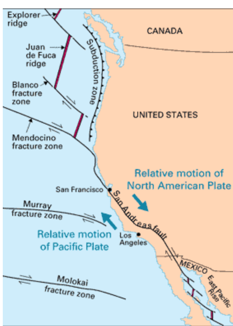
Plate Tectonic map of the western margin of North America. Notice that the San Andreas Fault connects offset portions of the Juan de Fuca ridge to the north with offset portions of the East Pacific Rise in the Gulf of California (or Sea of Cortez). There is still active subduction of the Juan de Fuca Plate in Northern California, Oregon, and Washington. In California, the San Andreas Fault System cuts through the continental plate, transferring some of the continental crust to the Pacific Plate, which is moving north towards Alaska and the subduction zones of the Aleutian Islands. © Prentice Hall Publishing
