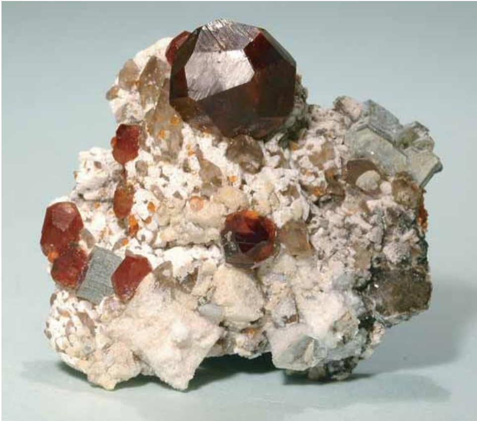
Figure 9. Photograph of a mineral specimen containing large crystals of the garnet mineral spessartine (red), showing the distinctive “euhedral isometric” crystal form of garnet. Used since ancient times for jewelry, the first industrial use of garnet was probably in coated sandpaper manufactured in the United States by Henry Hudson Barton in 1878. The United States currently consumes about 16 percent of the global production of industrial garnet. (Copyrighted photo by Stan Celestian/courtesy of Glendale Community College).
