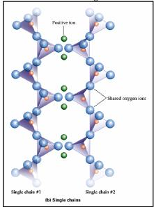
Amphibole family: **Hornblende** (Ca,Na)<sub>2-3</sub>(Fe,Mg,Al)<sub>5</sub>Si<sub>6</sub>(Si,Al)<sub>2</sub>O<sub>22</sub>(OH)<sub>2</sub> **Cleavage:** Two planes at 60° and 120°
