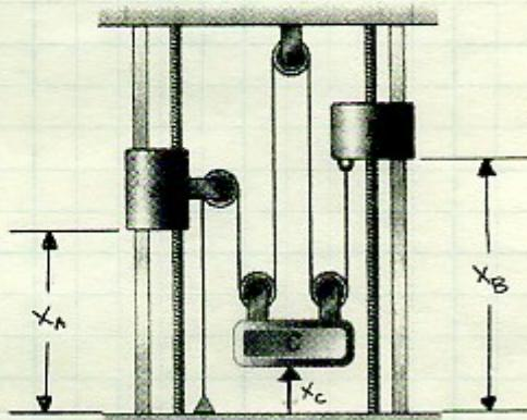
$$\begin{aligned} x_A + (x_A - x_c) + (-x_c) + (-x_c) + (x_B - x_c) &= \text{constant} \\ 2x_A + x_B - 4x_c &= \text{constant} \\ 2v_A + v_B - 4v_c &= 0 \\ 2a_A + a_B - 4a_c &= 0 \\ a_c &= 0.5a_A + 0.25a_B \quad \text{---(1)} \end{aligned}$$
