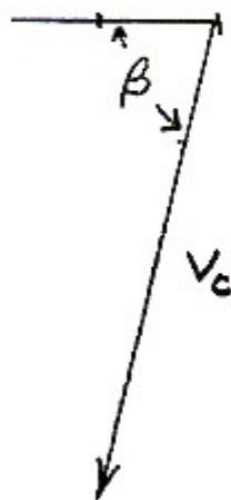
$$\begin{aligned} \text{Vertical motion: } (v_C)_y^2 &= [(v_C)_y]_0^2 - 2g(y - y_0) \\ &= (1.8 \sin 50^\circ)^2 - (2)(9.81)(-1.5) \\ &= 31.331 \text{ m}^2/\text{s}^2 \\ (v_C)_y &= -5.5974 \text{ m/s} \end{aligned}$$
