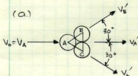
NOTE: After the collision, balls B and C move along the I.o.i. because there are no tangential forces. ( $v'_B$  and  $v'_C$  are as shown.)
