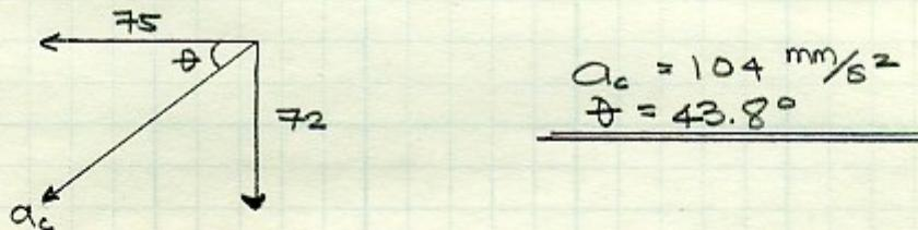
$$\begin{aligned}a_c &= 104 \text{ mm/s}^2 \\&\theta = 43.8^\circ\end{aligned}$$
