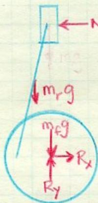
The only forces that do work are  $m_r g$  and  $m_f g$ . However,  $m_f g$  does not because the flywheel does not move.
