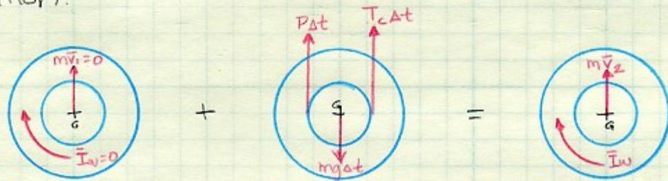
$$y: P\Delta t + T_c\Delta t - mg\Delta t = m\bar{V}_2$$
