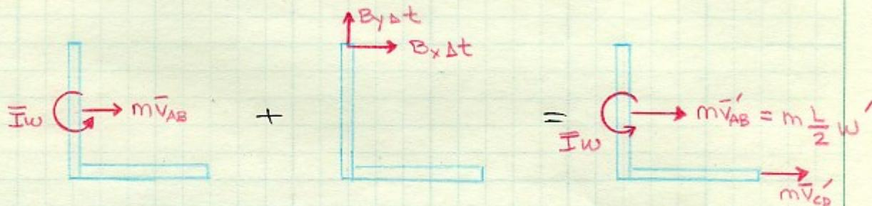
$$\begin{aligned} \omega &= \sqrt{\frac{3g}{L}} \\ \bar{I} &= \frac{1}{2} mL^2 \\ \bar{v}_{AB} &= \frac{1}{2} L \omega \\ &= \frac{1}{2} L \sqrt{\frac{3g}{L}} \end{aligned}$$
